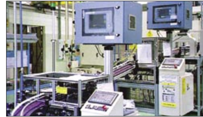
Uson systems are self-contained with integral material handling and data acquisition functions.
